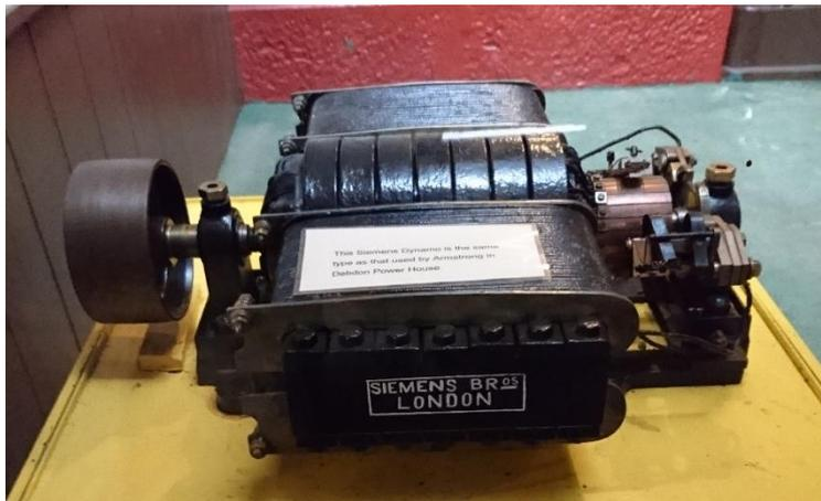
*Figure 1: Siemens dynamo installed at Cragside*
